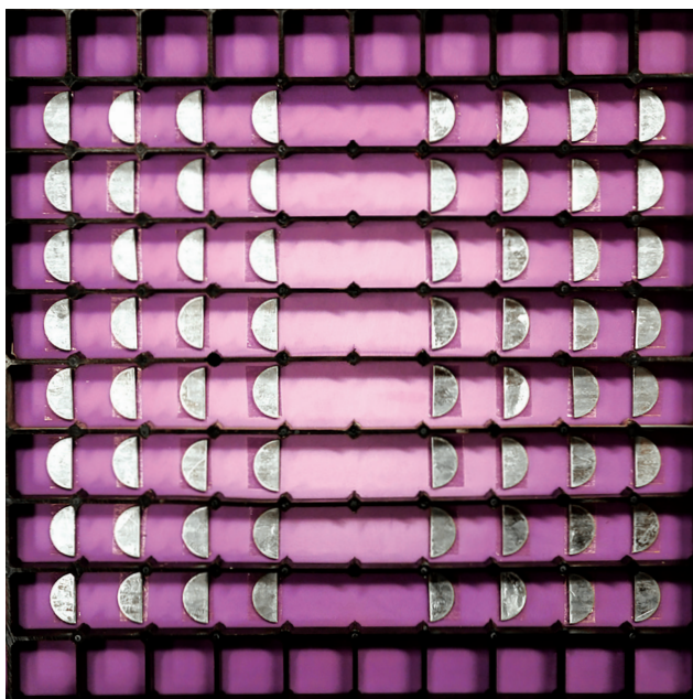
HKUST developed a thin, lightweight membrane-type acoustic metamaterial. The flimsy membrane, decorated by a button and backed by a shallow cell, could absorb more than 99% of low frequency sound.
